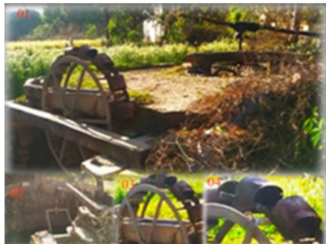
Figure 5: to draw water, a wheel with a chain of dolchi is installed in the well along with the operating device (01), the water level at the well depth (02), the structural design of the dolchi employed on the wheel (03 & 04).
